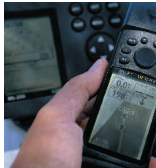
Figure 22 Global Positioning System (GPS) technology uses satellites to determine location on Earth's surface.
