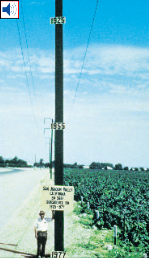
Figure 14 The years on the pole show how much the ground level dropped in the San Joaquin Valley, California, between 1925 and 1977.
